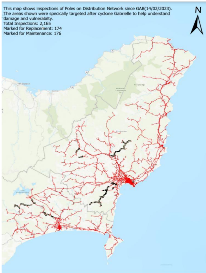
Screenshot 4: Map showing pole inspections arising from ariel review following Cyclone Gabrielle
