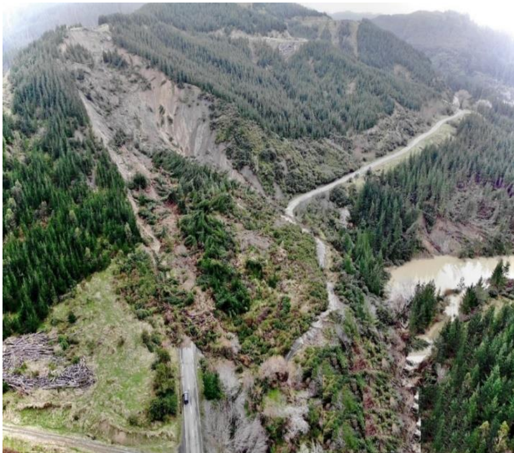
Photograph 2: Slip on Te Hau Road caused by heavy rains and a storm on 20 June 2024
